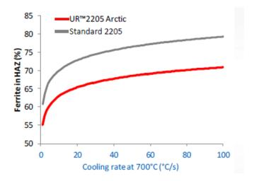
UR<sup>M</sup> 2205 Arctic can be welded either with the matching filler material (E2209) or with the overalloyed filler material (E2594). For gas processes, when a duplex wire is used a shielding gas with nitrogen addition  $(2\%N_2)$  is recommended to keep a satisfactory microstructure and appropriate corrosion resistance. For severe toughness requirements at low temperature (below -80°C), other filler materials can be recommended. *Please contact us.*
