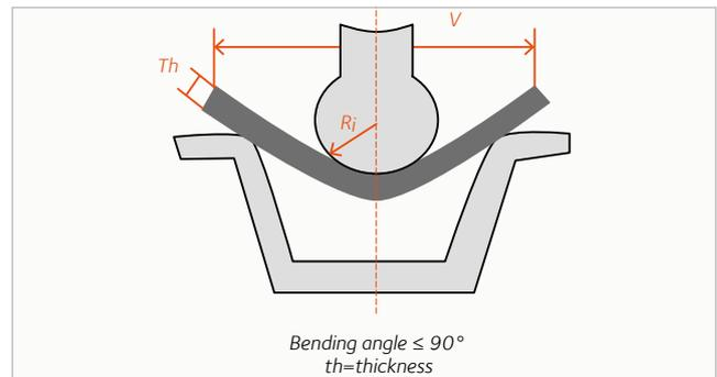
According above parameters, bending strength depends on bending length, thickness, die opening...
