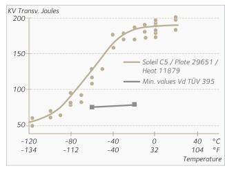
Soleil<sup>™</sup> C5 alloy presents improved toughness properties when compared to ferritic-martensitic grades (AlSI 410-420 / EN 1.4000-X6 Cr 13).
