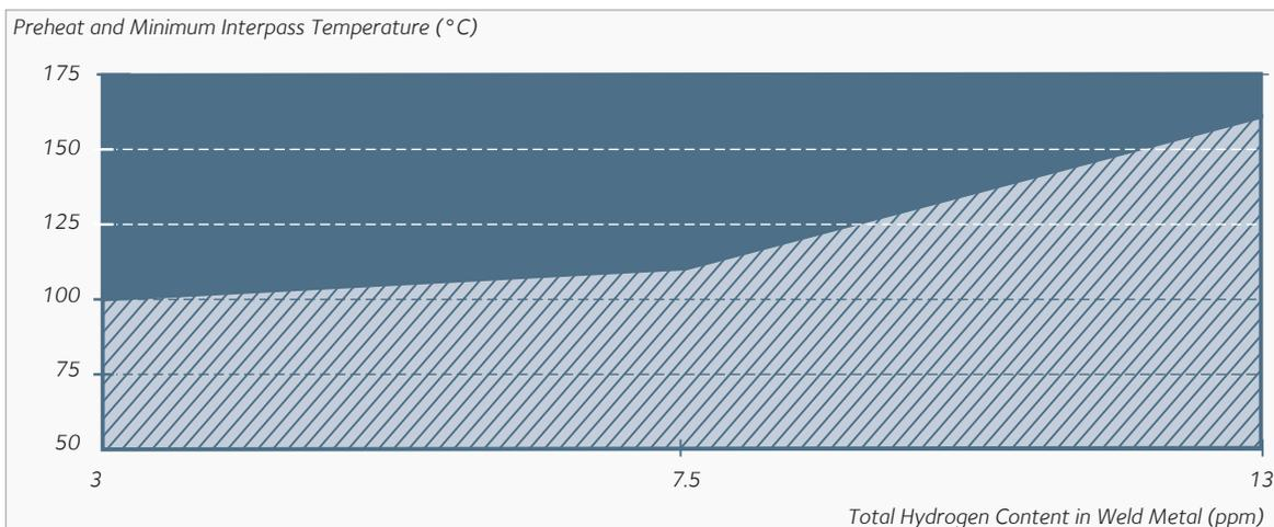
However, the risk of cold cracking is known to be greater in the weld metal than in the HAZ. Therefore, preheating and interpass temperatures of 200°C are recommended for thickness higher than 30 mm\*. After welding a Dehydrogenation Heat Treatment ≥ 300°C is recommended.
