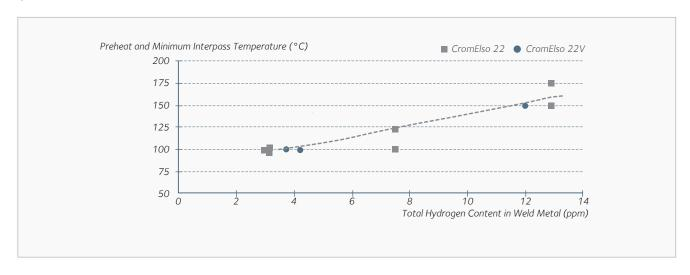
However, the risk of cold cracking is known to occur in the weld metal more frequently than in the HAZ. Therefore, a preheat and minimum interpass temperature of 200 °C is recommended for thickness higher than 30 mm\*. After welding a Dehydrogenation Heat Treatment  $\geq 300$  °C is recommended.
