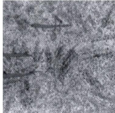
Homogeneous tempered bainite/martensite in prehardened condition (300 HB/32 HRC) Manganese sulfide inclusions (x 500).
