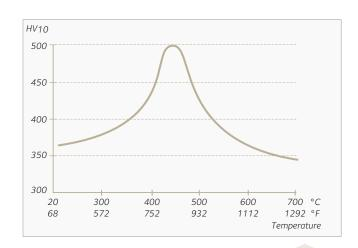
Hardness / Temperature tempered for 4 hours after austenitizing at 1040°C (1904°F) for 30 min. quenched 100°C/sec. (212°F/sec.).
