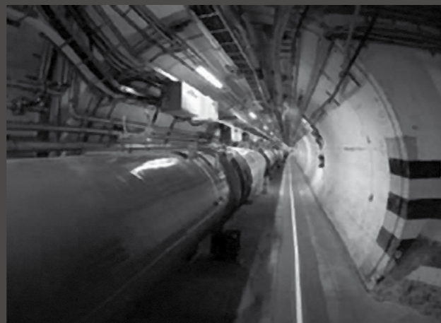
1.4429 Low ferrite content & magnetic permeability plates delivered for the super-conducting magnet half-shells (3000t, 41 km of half shells diameter 550 mm in 10.1 mm thickness)
